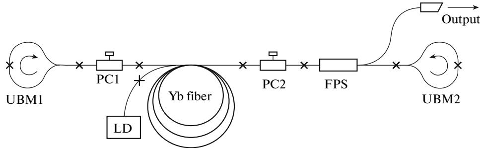
**Fig. 5.** Scheme of the proposed ultrashort-pulse ytterbium laser with the linear cavity and two ultrabroadband fiber reflectors: LD pumping laser diode, UBM1 and UBM2 ultrabroadband fiber mirrors, PC1 and PC2 fiber polarization controllers, and FPS fiber polarization splitter.
